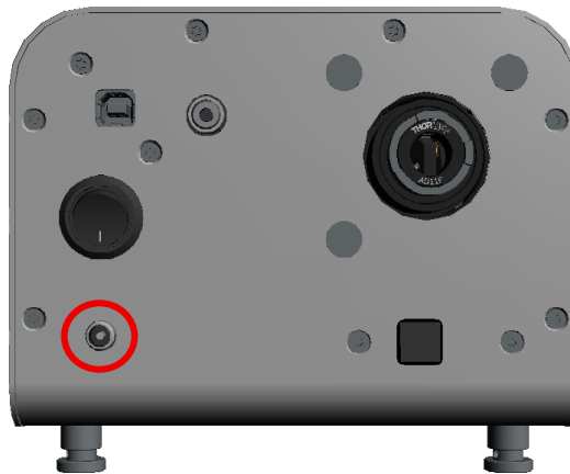
Fig 3. 24V Power Supply JACK connector.
